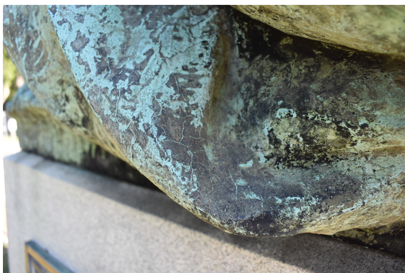
Fig. 12 - Crazing visible on what appears to be evidence of previous surface coating currently appearing as black - also seen in Fig. 11
