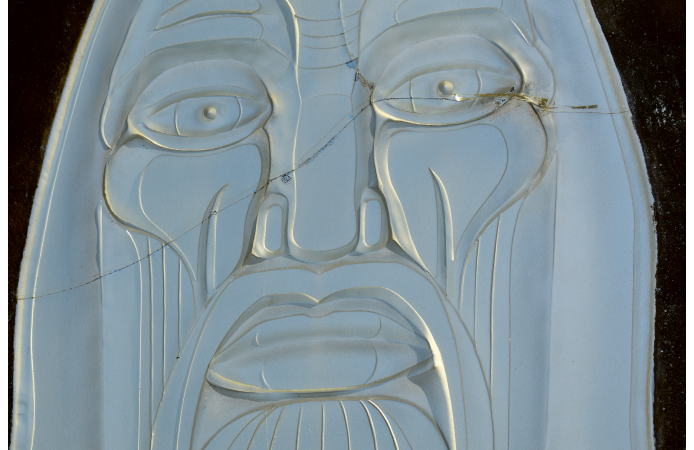
Fig. 9 - Moses interior detail showing network of cracks, corresponding spalling, and loss of "frosted" appearance in larger spalls
